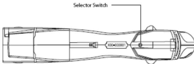
The selected mode displays for 5 seconds, and will be the default mode the next time the safety switch is moved to the up (ARMED) position.
