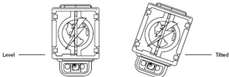
For most deployments, hold the CEW level. Do not tilt the CEW unless it is necessary to do so to align the CEW with the attacker.
