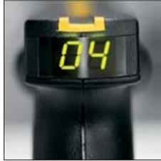
When the X26C CEW is deployed, it delivers an approximately 10-second Shaped Pulse™ energy burst of short-duration electrical impulses. The CID displays a countdown from 10 to 0 indicating how many seconds remain in the current burst. (The number 0 may be represented by 4 vertical lines instead of a number.) The burst can be stopped at any time by shifting the safety switch to the down (SAFE) position.
